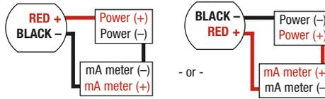
If the 4-20 mA analog output is not required, the transmitter will function as a low voltage powered pressure gauge when connected to any 8 to 32 VDC power supply. Connect the loop (+) supply to the RED lead and the loop (-) supply to the BLACK lead.
